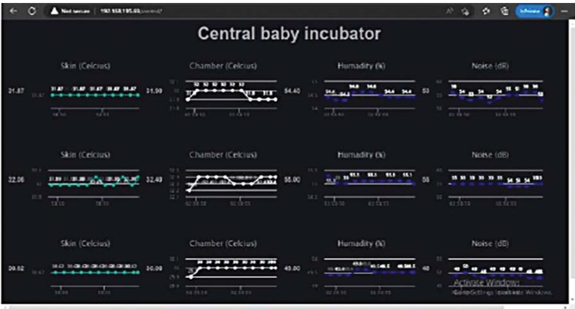
Fig. 3. The display screen displays the investigated incubator parameters in real time
