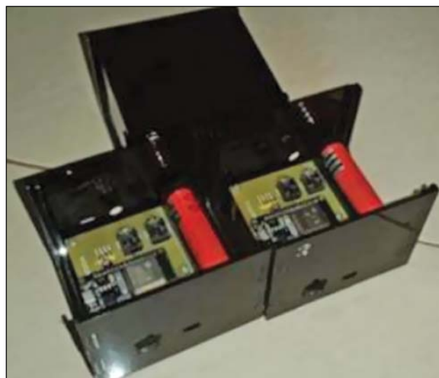
Fig. 2. The design of the module for monitoring the parameters of the newborns' incubator
